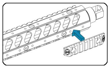
1 Install the rail on the handguard in the desired position
