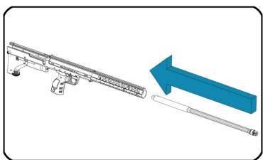
Gently insert the barrel inside the receiver.
