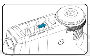
6 Make sure the tab is in the locked position (toward the receiver)
