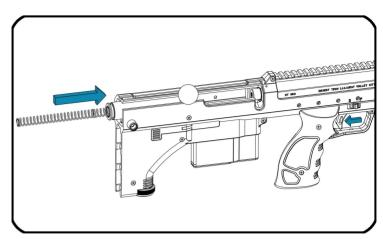
While the trigger is pulled back, slide the bolt head, the cylinder assembly, the piston & spring inside the receiver.
