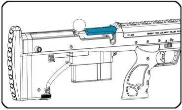
3 Push the bolt foward to compress the spring and engage a bb inside the hopup (you can visualy check inside the hopup if your magazine is empty).
