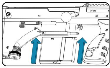
2 Insert the magazine firmly to ensure correct magazine retention.
