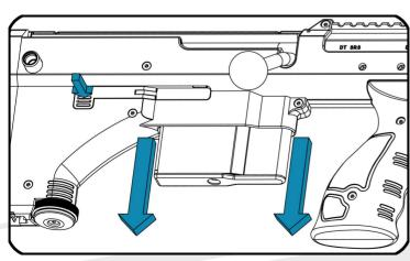
**3** To remove the magazine, pull the magazine down after depressing the right side magazine release button.
