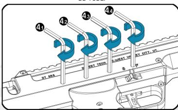
A Secure the barrel by tightening the 4 barrel screws, from bolt to muzzle side (and reverse order for removal).
