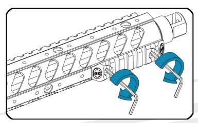
2 Secure the rail using two M4x10 screws from the screw set bag.
