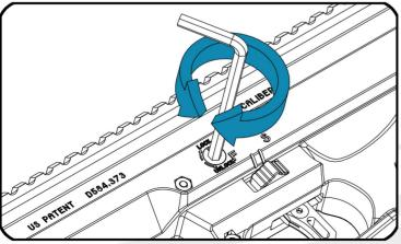
3 Set the barrel lock to «LOCK» position.
