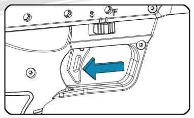
Pull the trigger to release the spring guide inside the buttplate.
