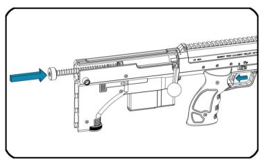
**3** While the trigger is still pulled back, insert the spring guide inside the spring, then push it into the receiver.
