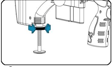
3 For fine-tune adjustments, turn the monopod knob clockwise to add elevation and counter-clockwise to decrease elevation.
