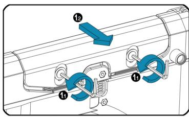
Loosen the two M5x6 screws.
