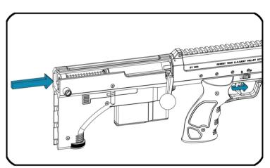
4 After pushing the spring guide inside the receiver, release the trigger and push it forward. Keep forward pressure on the trigger in order to lock the spring guide inside the receiver.
