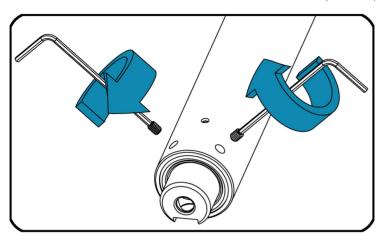
① Install the two hopup screws (M3x4) from the screw set bag. ⚠ If you're using long knurled hopup screws, you have to assembly the barrel inside the gun before to assembly hopup screws
