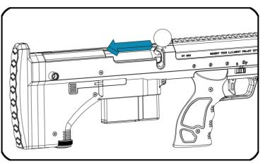
2 Move the bolt backward to compress the spring and lock the piston sear (until it clicks).
