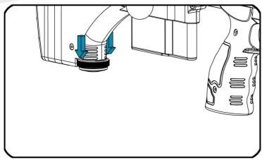
1 To release the monopod, pull down on the monopod knob.
