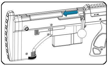
5 Insert the dust cover into the ejection window, then slide it backward.
