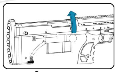
1 Pull up the bolt handle. A Make sure that the bolt is not already armed to avoid double feed.
