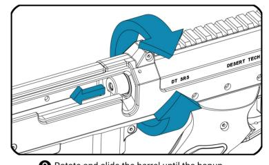
Rotate and slide the barrel until the hopup fits onto the BB-tube.
