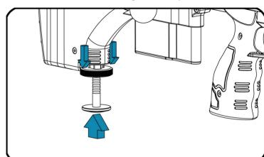
To return to original retracted position, push up on the monopod foot while holding the monopod knob downward.
