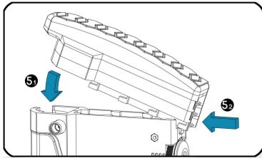
While the trigger is still pushed front, slide buttplate starting at the bottom and sliding up.
