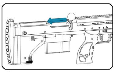
2 Move the bolt backward to engage the piston end on the piston sear (until it clicks).
