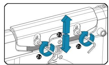
Adjust the cheekpad position (six positions allowed). Tighten the two M5x6 screws to lock the position of the cheekpad.
