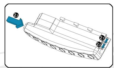
To remove a buttplate spacer, while pressing the tab backward, push the buttplate downward Repeat this to remove two layers.
