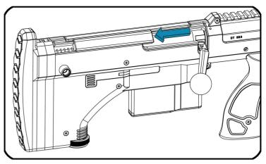
8 Insert the dust cover into the ejection window, then slide it backward.
