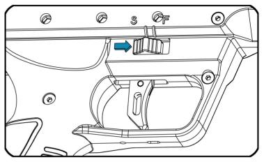
2 Slide the safety button (right or left) to «F» position to disengage the safety.
